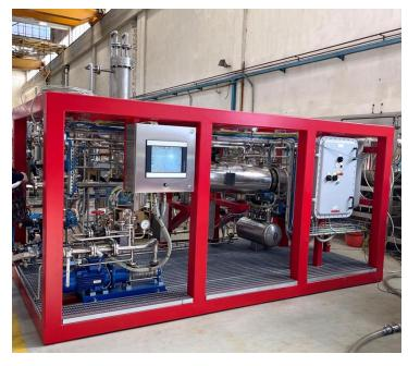
separation of liquid solvents, this adaptable system allows users to tailor it to their unique separation requirements effortlessly. The versatility of the system enables testing of membranes across various modules, providing a comprehensive assessment of their stability and performance in separation processes. A key feature of the system is its capability to operate in three distinct membrane process, enhancing its flexibility and applicability.
