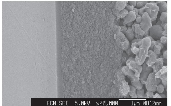
Cross-sectional SEM micrograph of the layered structure of a hybrid membrane, showing the supporting layers and the ~150 nm thick selective HybSi® top layer.
