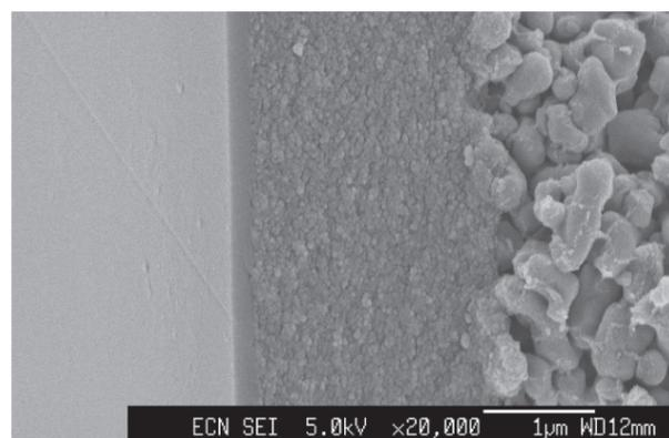
Cross-sectional SEM micrograph of the layered structure of a hybrid membrane, showing the supporting layers and the ~150 nm thick selective HybSi® top layer.
